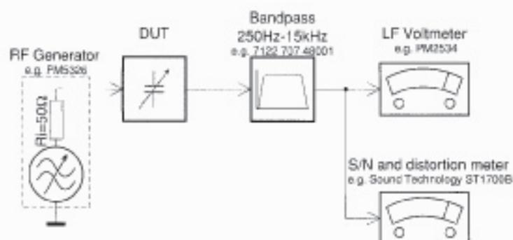
Use a bandpass filter to eliminate hum (50Hz, 100Hz) and disturbance from the pilotone (19kHz, 38kHz).
