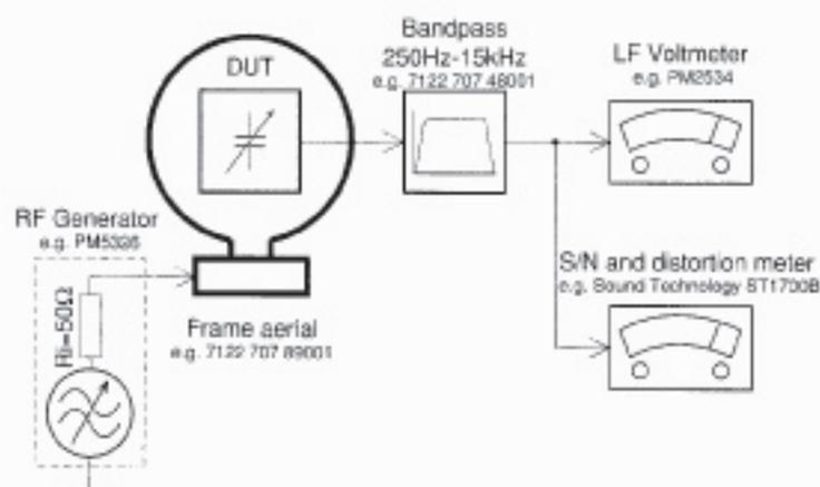
To avoid atmospheric interference all AM-measurements have to be carried out in a Faraday's cage. Use a bandpass filter (or at least a high pass filter with 250Hz) to eliminate hum (50Hz, 100Hz).
