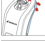
now push right on the housing and left on the cover so you can remove the cover.
