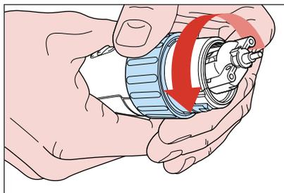
Turn the zoomring (7), till the combholder (6) is on its highest position. After that, go on turning the zoomring (7), with a little bit more force, till the combholder (6) comes out of his seat.
