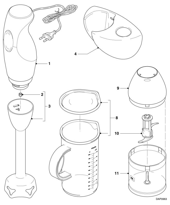
power unit 1 speed rubber ring metal bar wall holder beaker and lid chopper gear box chopping knife chopping bowl West Europe
