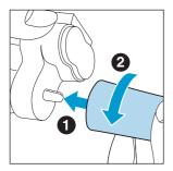
Turn the toothbrush upside down and press it down on a hard surface to remove the battery holder.
